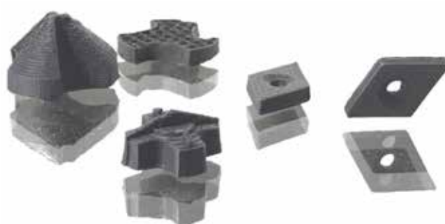
Fig. 4. Geometries of cutting tools that can be realized by 3D shaping of MEAM.
