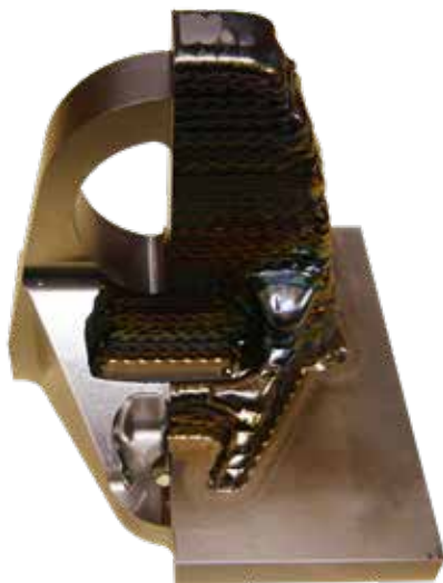
Fig. 2. Printed bearing bracket made of Ti64 with partial machining.
