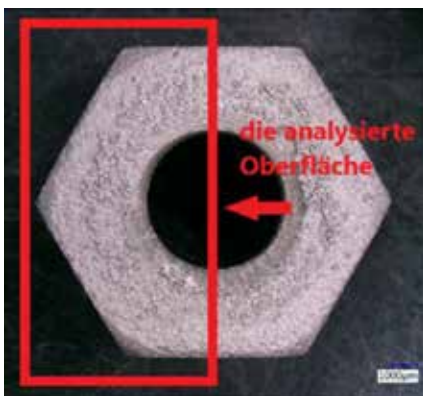
Fig. 12. The nut was cut in the area marked in red for the cross-section.
