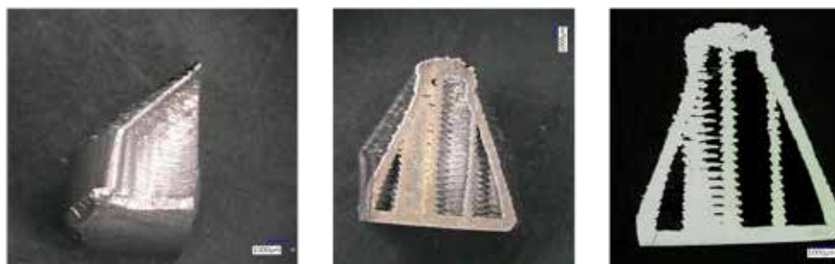
Fig. 6. Cross sections of cut sintered MEAM parts with hollow structures internally.
