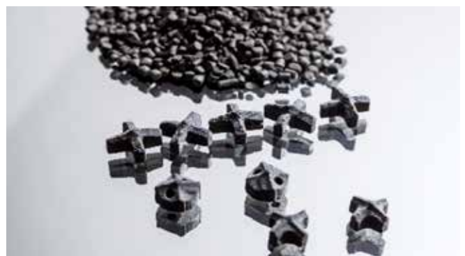
Fig. 1. WC-Co parts printed from granules by the indirect 3D technology material extrusion additive manufacturing.
