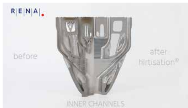
Fig. 2. Cross-sections of a manifold used in automotive applications. The printed part (left) includes internal support structures that cannot be removed mechanically. In the finished part the support structures have been completely removed and the surface levelled. (Hirtisation® treatment, picture courtesy of RENA Technologies Austria)
