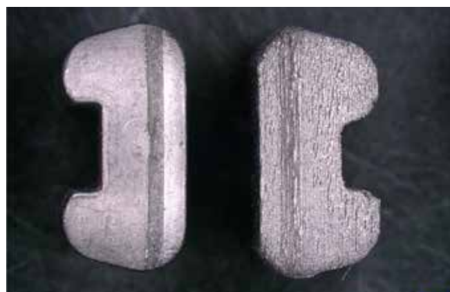
Fig. 5. Injection-moulded sintered hard metal part (left); MEAM 3D-printed and sintered hard metal part (right).
